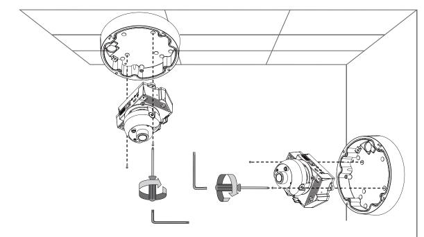
**Step 5** Secure the IP camera to the conduit base with two included screws.
